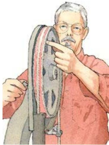
Turning the tracking adjustment in adjusts the blade toward the back of the wheel.
